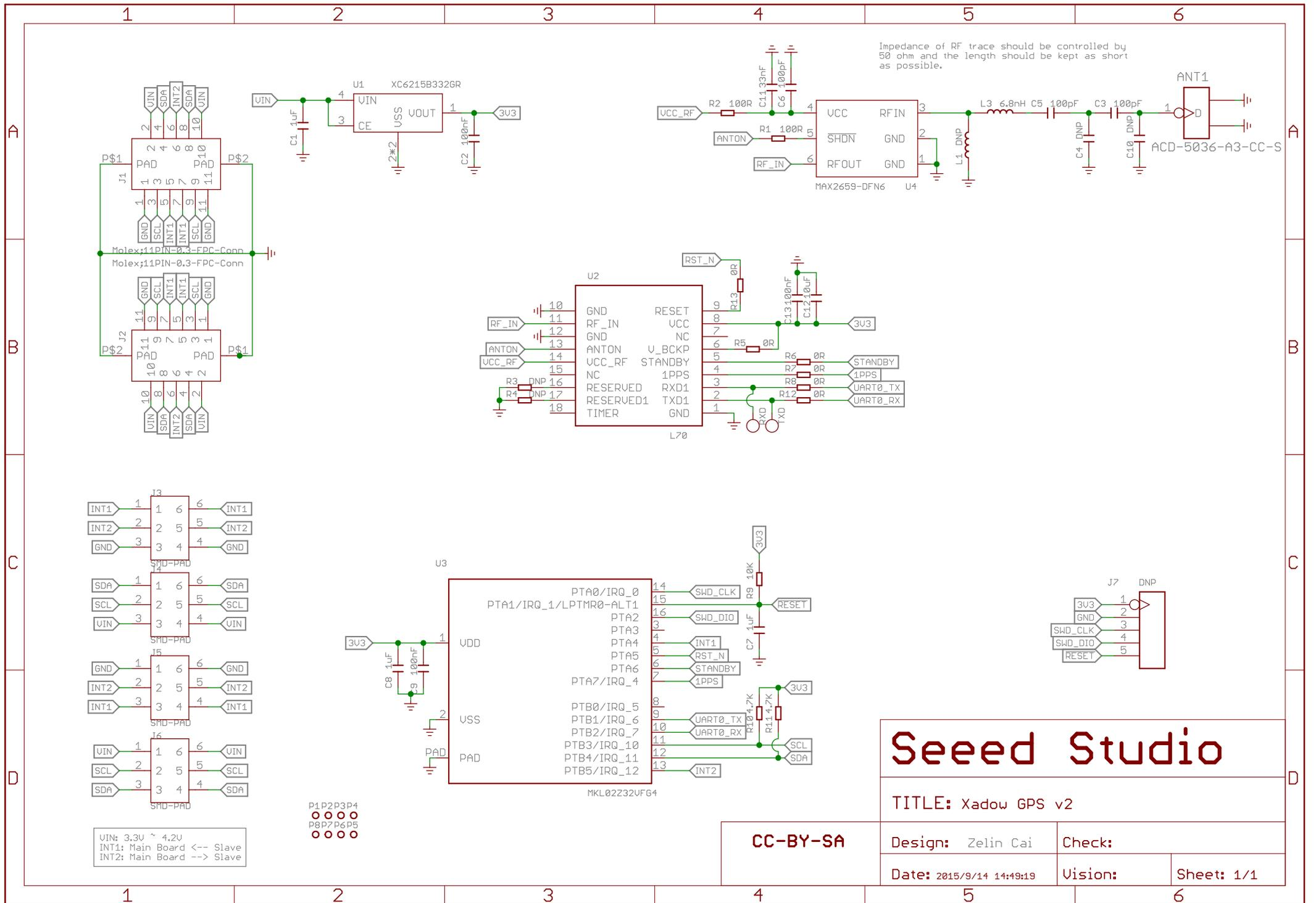
Impedance of RF trace should be controlled by 50 ohm and the length should be kept as short as possible.
