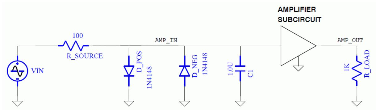
Figure 26.2: Example Circuit 2
