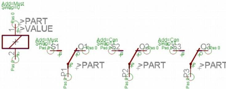
➤ *Relay with one coil and three contacts*
