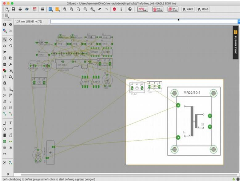
➤ **Board command: Create the layout from the schematic**
