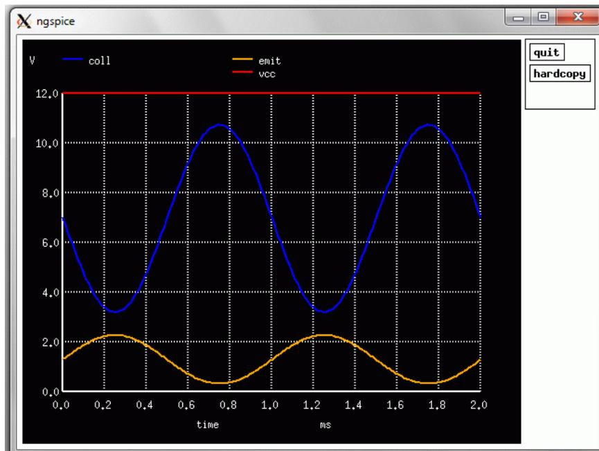
Figure 21.3: VCC, Collector and Emitter Voltages
