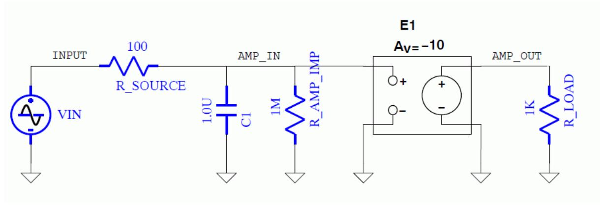
Figure 26.1: Example Circuit 1
