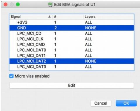
The dialog shows the list of signals connected to the BGA.
