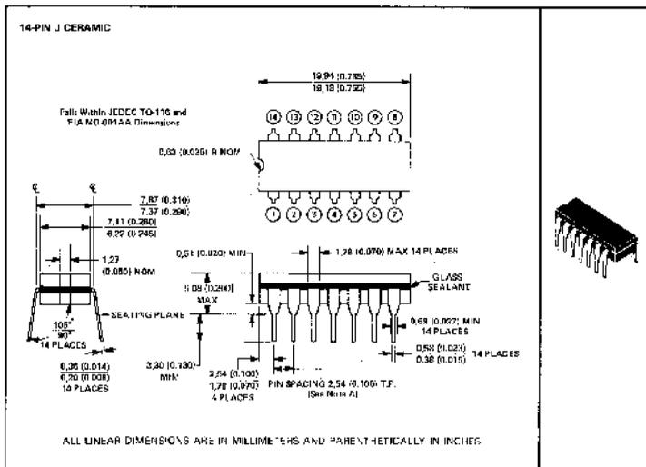
NOTE A: Each pin centerline is located within 0.28 (0.011) of its true longitudinal position.
